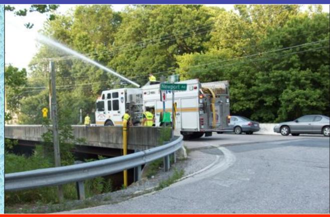
The standpipe is easily deployed by one or two persons. A 1,500 gpm pumper is shown here drafting from the deployed standpipe. A flow of 1,000 gpm+ was obtained.
